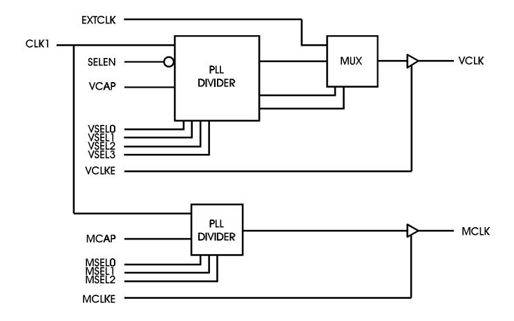
Figure 2-2 ICS90C61A Functional Block Diagram
