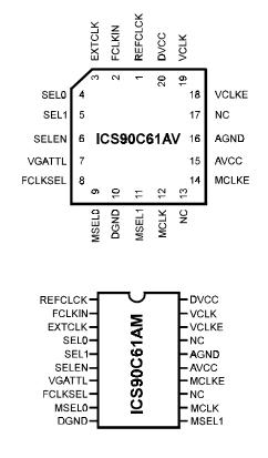
Note: ICS90C61AN (DIP) pin-out is identical to ICS90C61AM (SOIC) pin-out.
