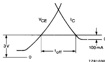
The turn-off time is the time taken for  $I_C$  to decrease to 100 mA after  $V_{CE}$  has risen 3 V into its flyback position.
