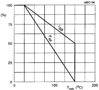
Fig.9 Power derating and second breakdown current curves.
