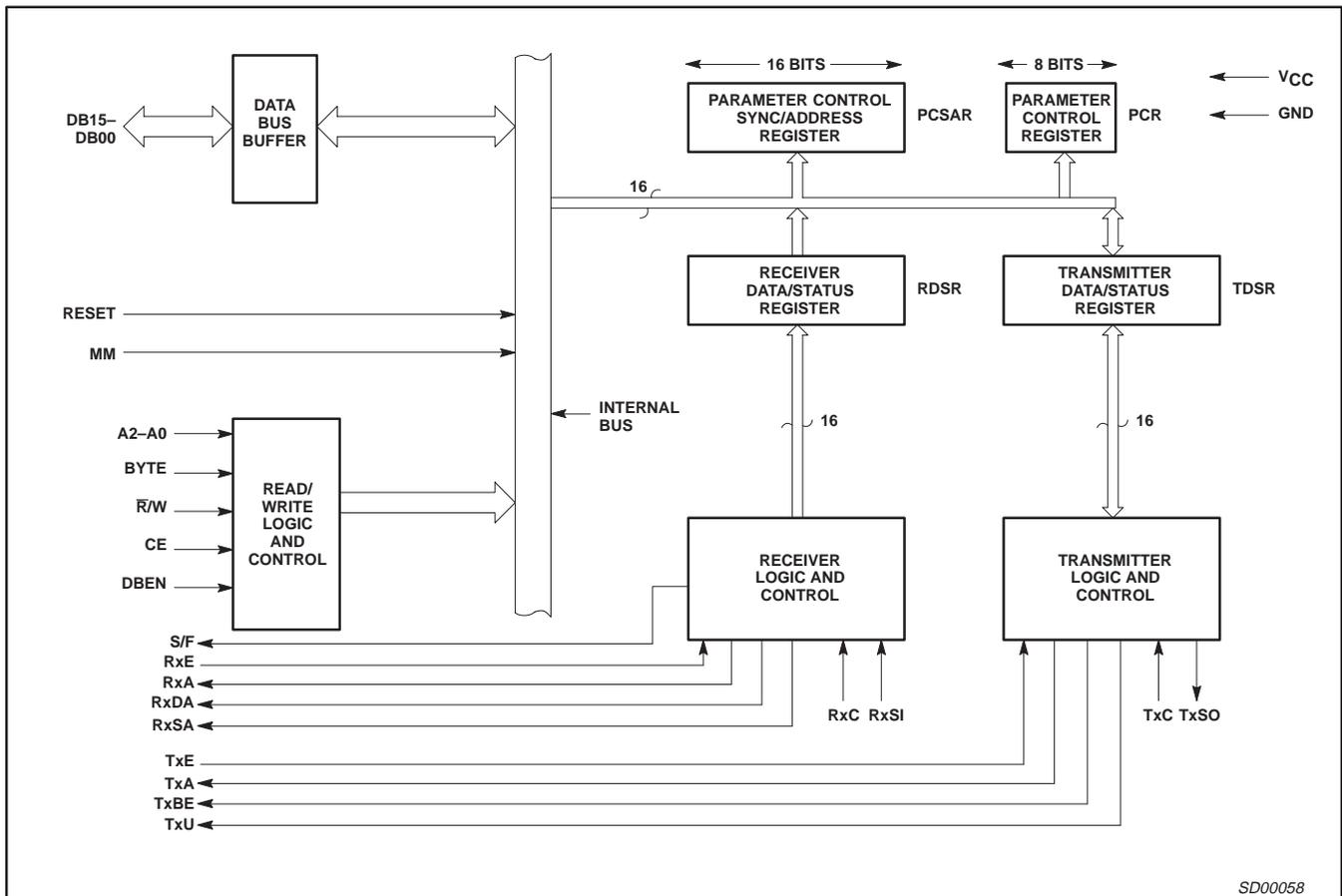
Figure 2. Block Diagram
