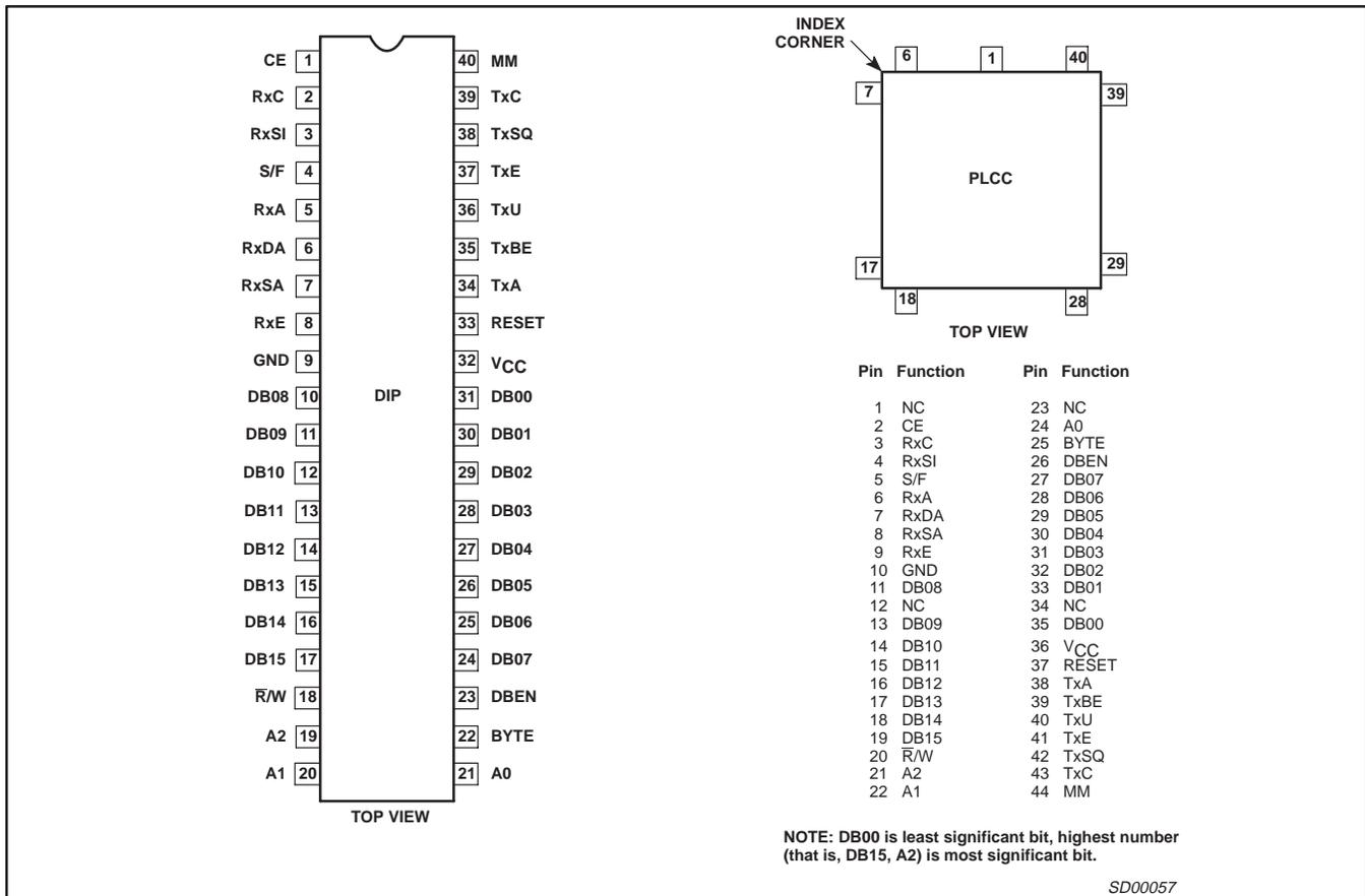
Figure 1. Pin Configuration
