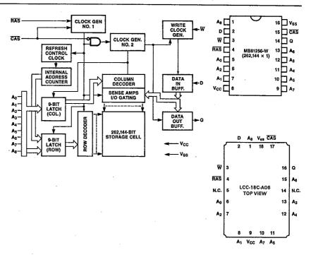
Note: The following IEEE Std. 662-1980 symbols are used in this data sheet:  $D = Data In, \overline{W} = Write Enable, Q = Data Out.$
