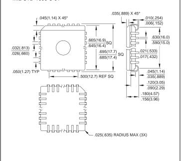
**44LW**, 44-Pad, Windowed, Ceramic Leadless Chip Carrier (LCC)
