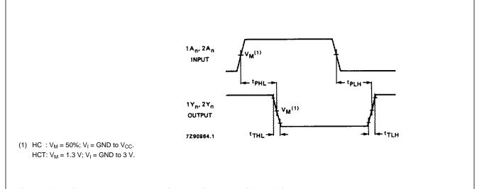
Fig.5 Waveforms showing the input  $(1A_n, 2A_n)$  to output  $(1Y_n, 2Y_n)$  propagation delays and the output transition times.
