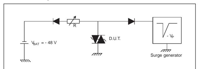
This is a GO-NO GO test which allows to confirm the holding current (I<sub>H</sub>) level in a functional test circuit.
