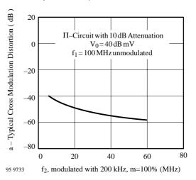
Figure 3. Typ. Cross Modulation Distortion vs. Frequency f<sub>2</sub>
