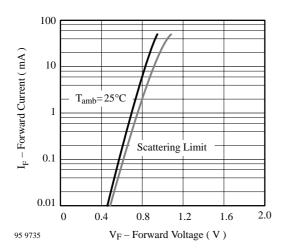
Figure 1. Forward Current vs. Forward Voltage
